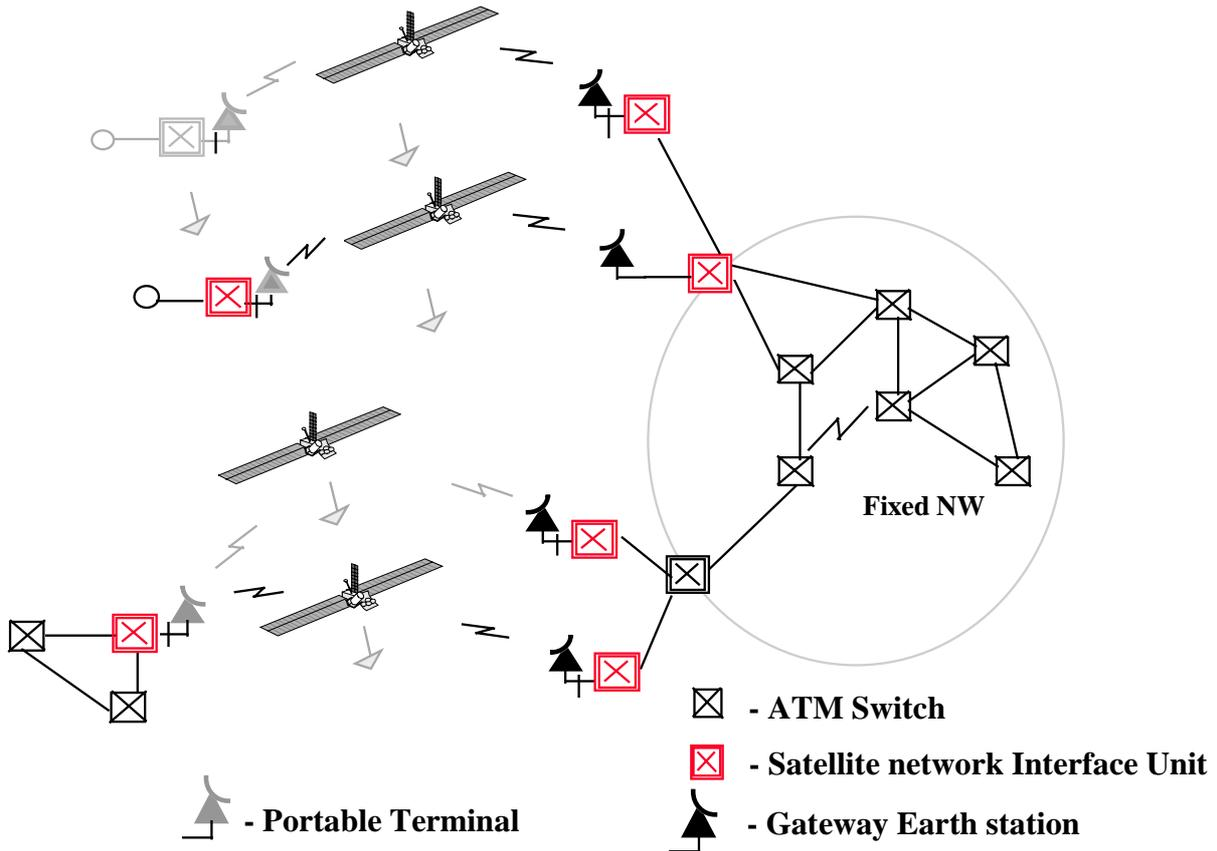
**FIGURE 6-1 LEO SATELLITE NETWORK USING REPEATER SATELLITES**
