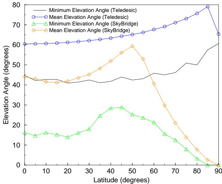
**FIGURE 4-21 MINIMUM AND MEAN ELEVATION ANGLE FOR SKYBRIDGE AND TELEDDESIC**
