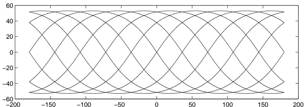
**FIGURE 4-10 EXAMPLE ROSETTE GROUND TRACK (SKYBRIDGE 80-SATELLITE APPROXIMATION)**
