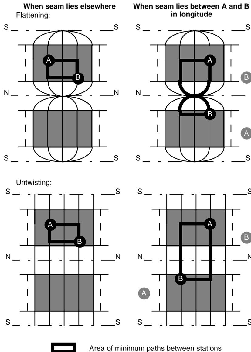
**FIGURE 4-13 HOW SEAM DISTANCE VARIES APPARENT NETWORK DISTANCE**
