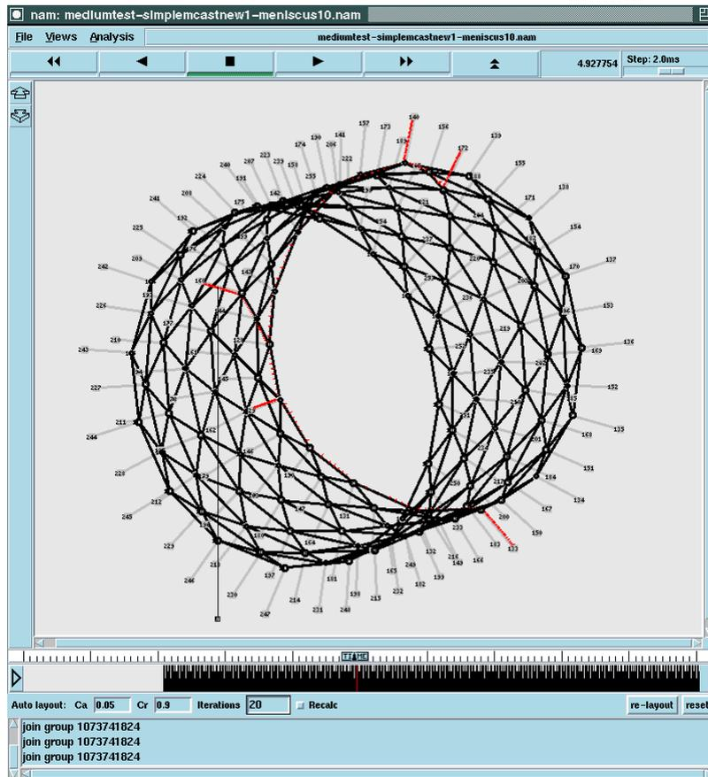
**FIGURE 4-15 SIMULATION OF SIXWAY CONNECTIVITY FOR 8/18/2 CONSTELLATION**
