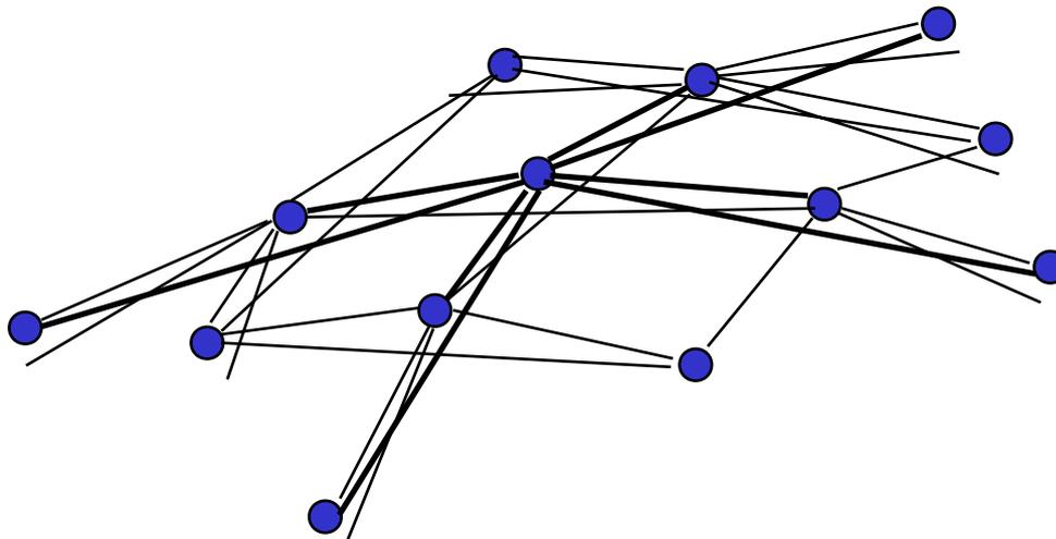
**FIGURE 4-20 PART OF TELEDDESIC NETWORK MESH SHOWING DUAL NETWORK DIVERSITY**
