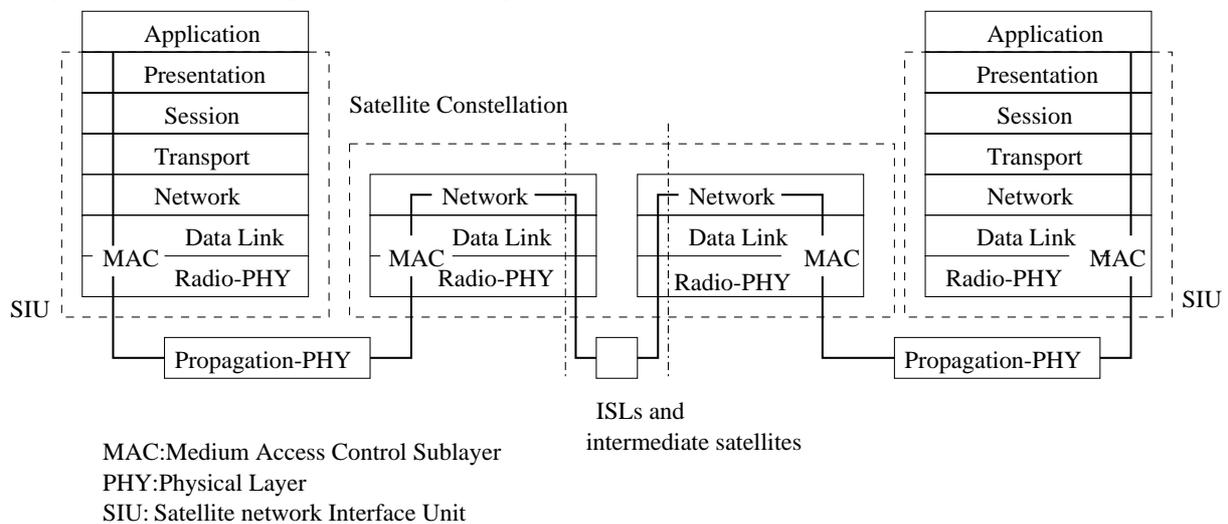
**FIGURE 4-18 ISL ROUTING APPROACH A LA TELEDDESIC**
