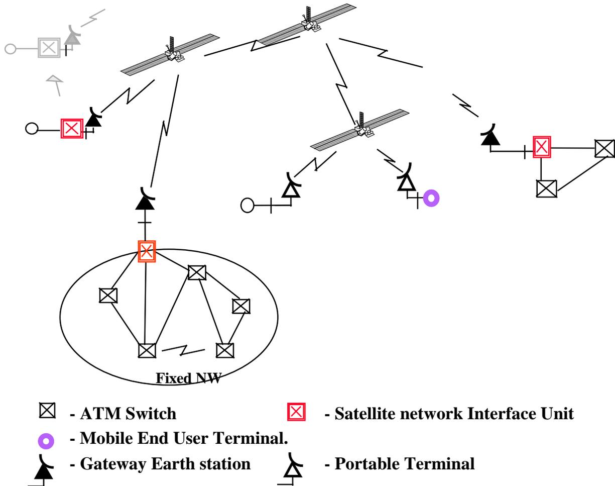
**FIGURE 6-2 LEO SATELLITE NETWORK USING ON-BOARD SWITCHING SATELLITES**
