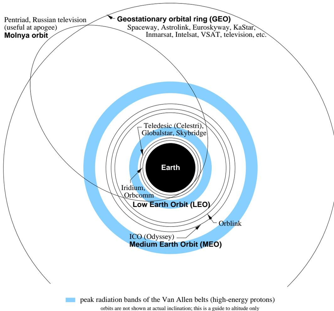
**FIGURE 4-4 ORBITAL ALTITUDES FOR SATELLITE CONSTELLATIONS**
