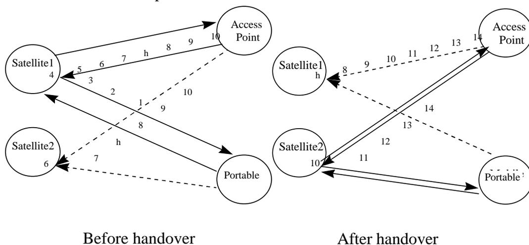
**FIGURE 4-25 HANDOVER PROCEDURE, DIFFERENCE IN PROPAGATION DELAYS**
