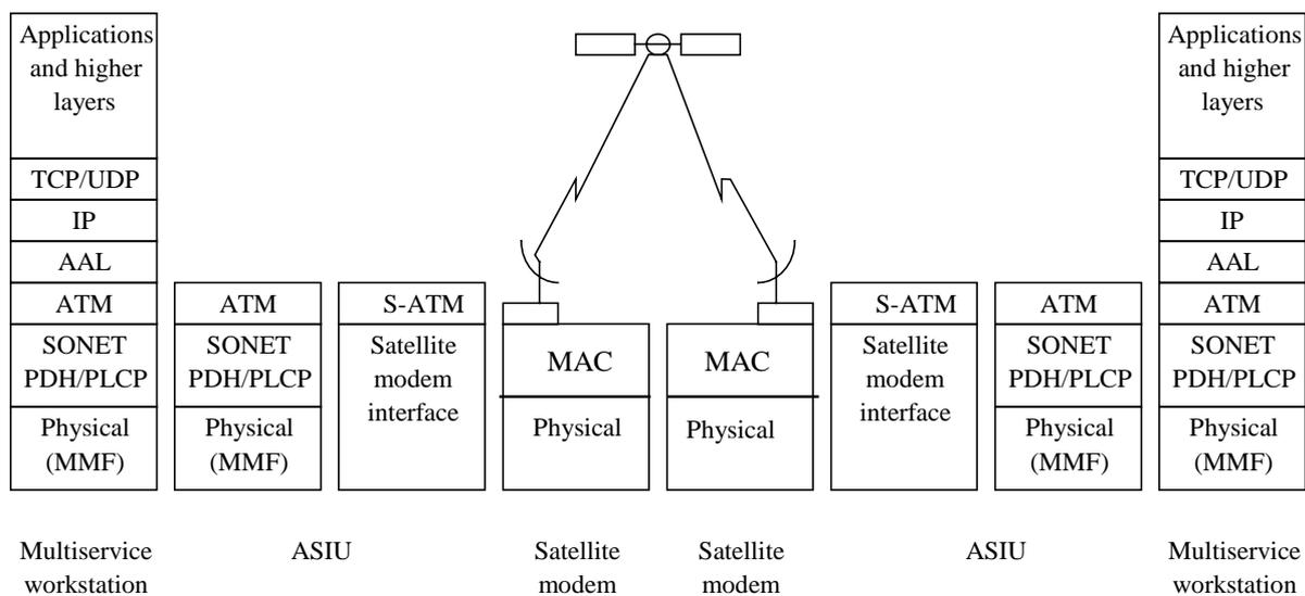
**FIGURE 2-1 PROTOCOL STACK FOR THE SKYBRIDGE SATELLITE ATM NETWORK**
