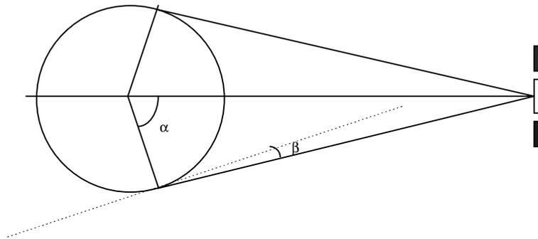
**FIGURE 4-23 RELATION BETWEEN ELEVATION ANGLE AND ALTITUDE**
